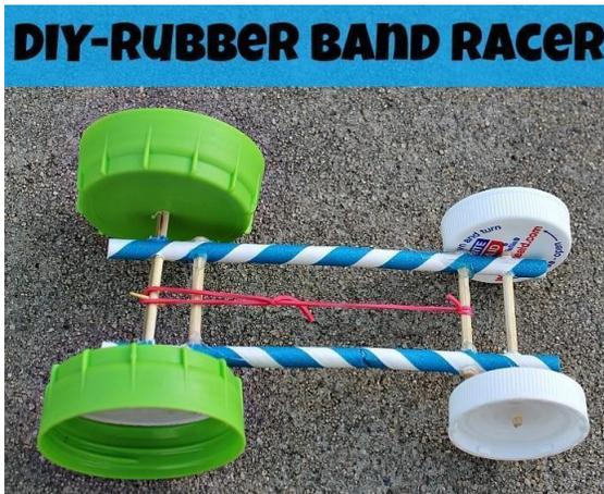
Step 1: Bore hole in two straws that are placed in parallel lines, and insert the toothpick or small piece of wood through these two holes and secure it (this is the inner stick)
